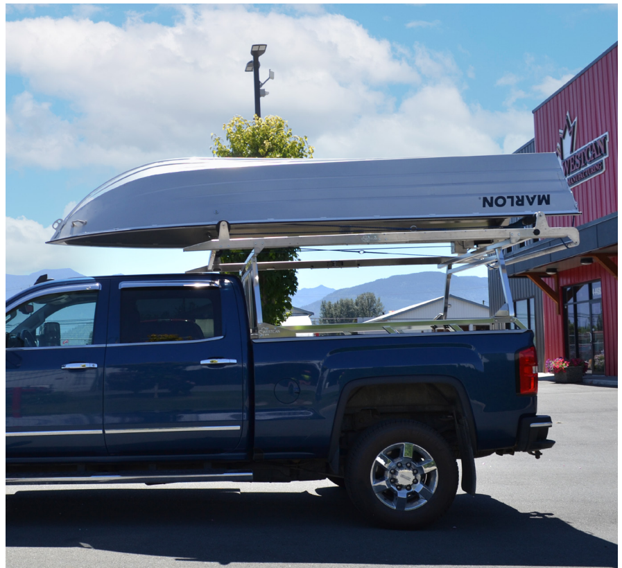
On the Fly Boat Loader installed on a Westcan Cab Guard, Rail Caps, Rear Rack and Truck Rack Extenders
